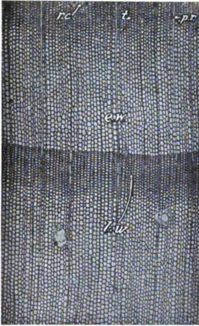
FIG. 3. — Transverse Section of Norway Pine. Magnified 25 Diameters. (Bull. 139, U. S. For. Ser.)
